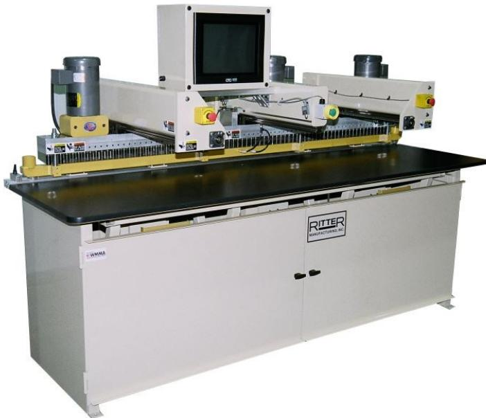
The Ritter R76 is a closet system drill part of the panel master series. The R76 is a CNC single row system drill with programmable drill row location and boring depth. The R76 is used for drilling full length closet panels in a single process. The drill row ball screws and linear rails provide for precision drill row location. The servo driven ball screw table feed control allows for precision drill depth control and through feed boring.
